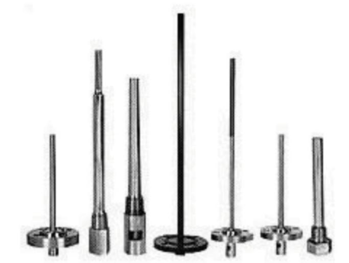
Thermowell allows removing / replacing of sensor without shutting down the process. This can be made from materials like SS 304, 316, 304L, 316L, 310, 446, Carbon Steel, Hestalloy.C, Monel.
